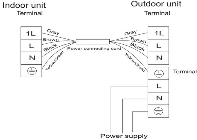
For these models, the power supply are connected from outdoor unit, with a circuit breaker.
