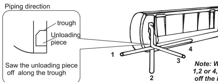
*Note: When installing the pipe at the directions 1, 2 or 4, saw the corresponding unloading piece off the indoor unit base.*
