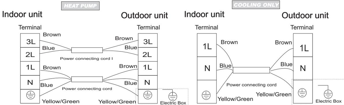
For above models, the power supply are connected from indoor unit.
