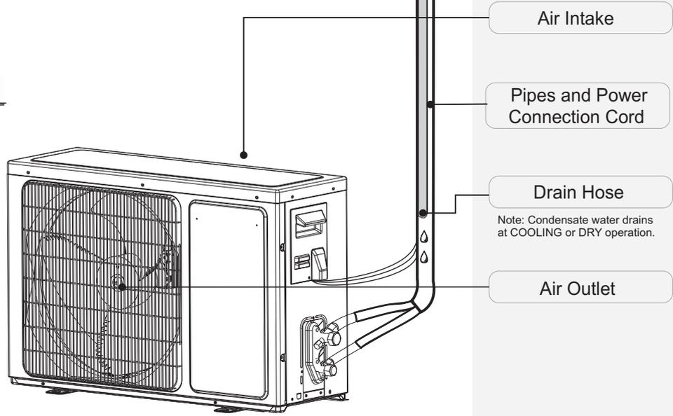
Note: Condensate water drains at COOLING or DRY operation.
