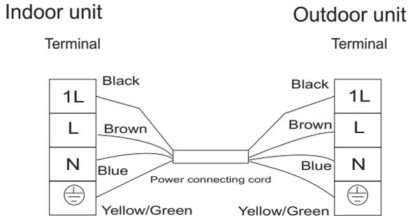
For these models, the power supply are connected from indoor unit.
