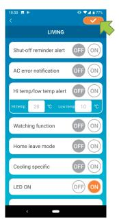
Switch between [ON] and [OFF], and tap on the top right of the screen to save the settings you changed.
