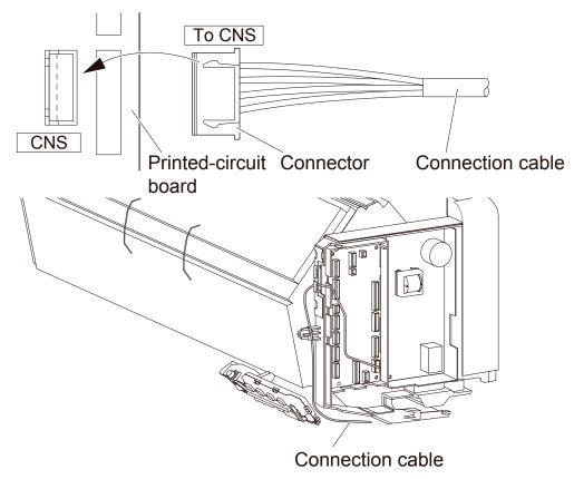
Connect the indoor unit connection cable to the indoor control printedcircuit board.
