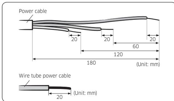
3 Insert both sides of core wire of the power cable into the connection sleeve.
