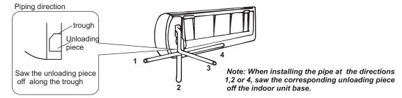
After connecting piping as required, install the drain hose. Then connect the power cords. After connecting, wrap the piping, cords and drain hose together with thermal insulation materials.
