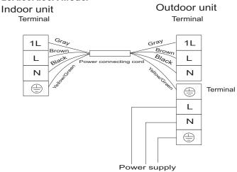
For these models, the power supply are connected from outdoor unit, with a circuit breaker.
