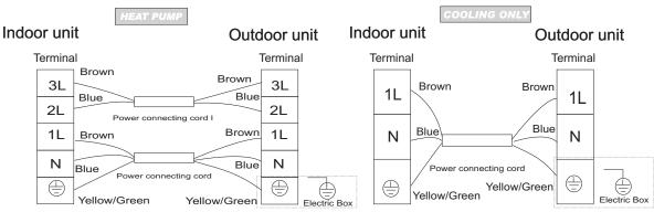
For above models, the power supply are connected from indoor unit.
