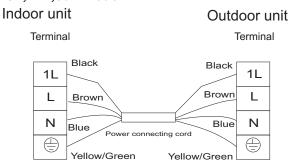
For these models, the power supply are connected from indoor unit.
