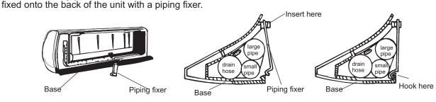
A. Insert the pipe fixer to the slot.
